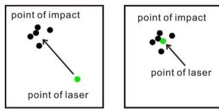
5. Take aim again using the exact same sight picture as in step#4. Turn on the laser sight and you will see the difference in distance between the laser dot and the real point of impact. To adjust the laser to be point of impact the windage and elevation will need to be adjusted. Rotating the windage and elevation with Allen wrench to adjust the laser.
