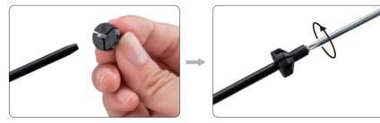
2. Make Sure that our bore sight tool is inserted deeply into the barrel's breech chamber to achieve a snug fit.
